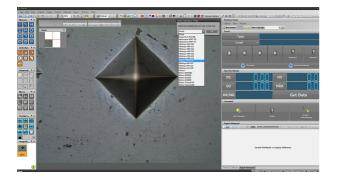
With the measurement tools of iWorks EX, iWorks HL is the basic version software for hardness test machine. You can measure the penetrator from Micro-Vickers, Vickers, Brinell under various standard selection.
